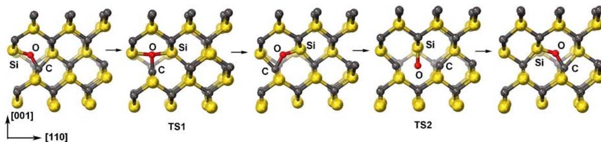
Fig. 2. The geometrical configuration of atoms corresponding to 5 ground states (3 energy minimums and 2 saddle points TS1 and TS2) during the migration of an oxygen atom in SiC-3C in the [110] direction for one lattice period of 3.08 Å. Atoms Si, C, O are signed by letters
